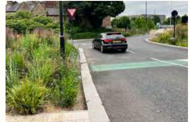
Rain gardens within the street network help to reduce water run-off
