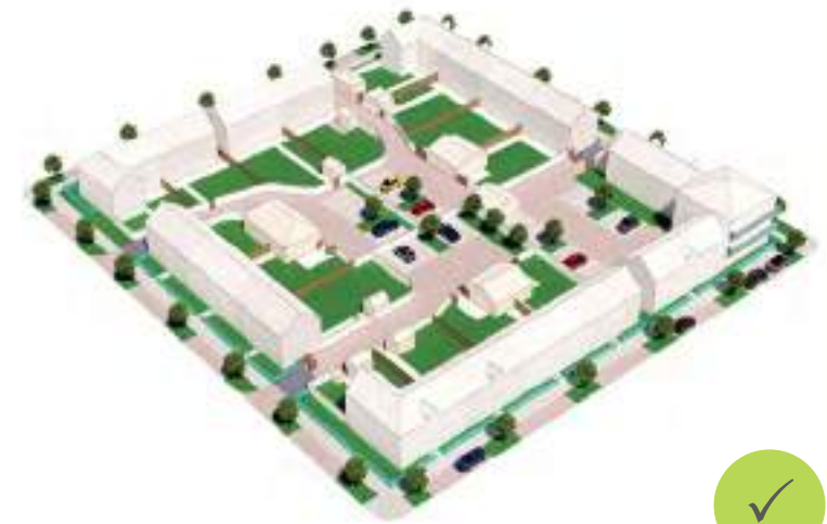
Perimeter block with mews development and parking overlooked by homes and Flats Over Garages
