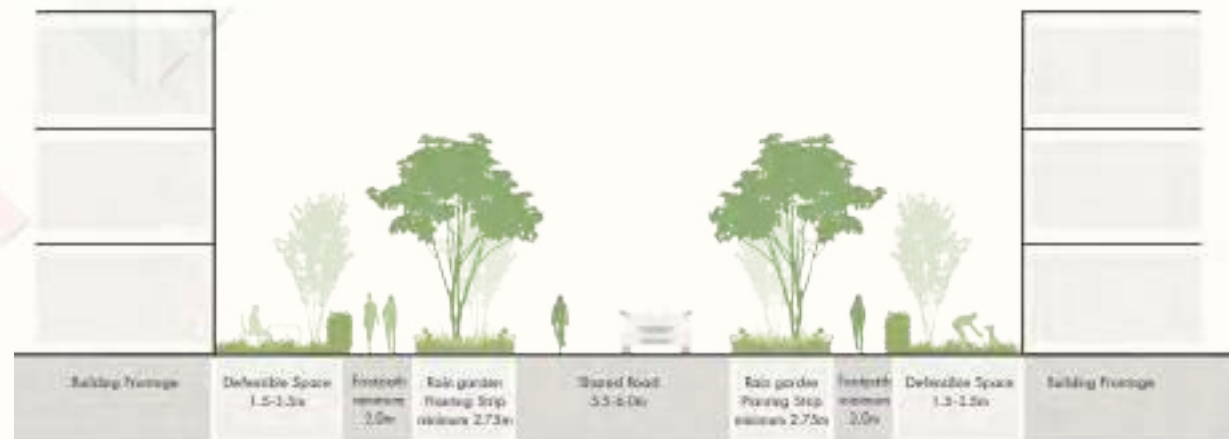
Indicative Secondary Street Section
