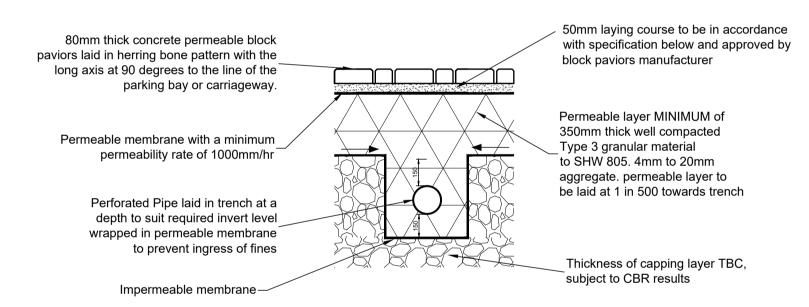
**Type C Permeable Paving**
