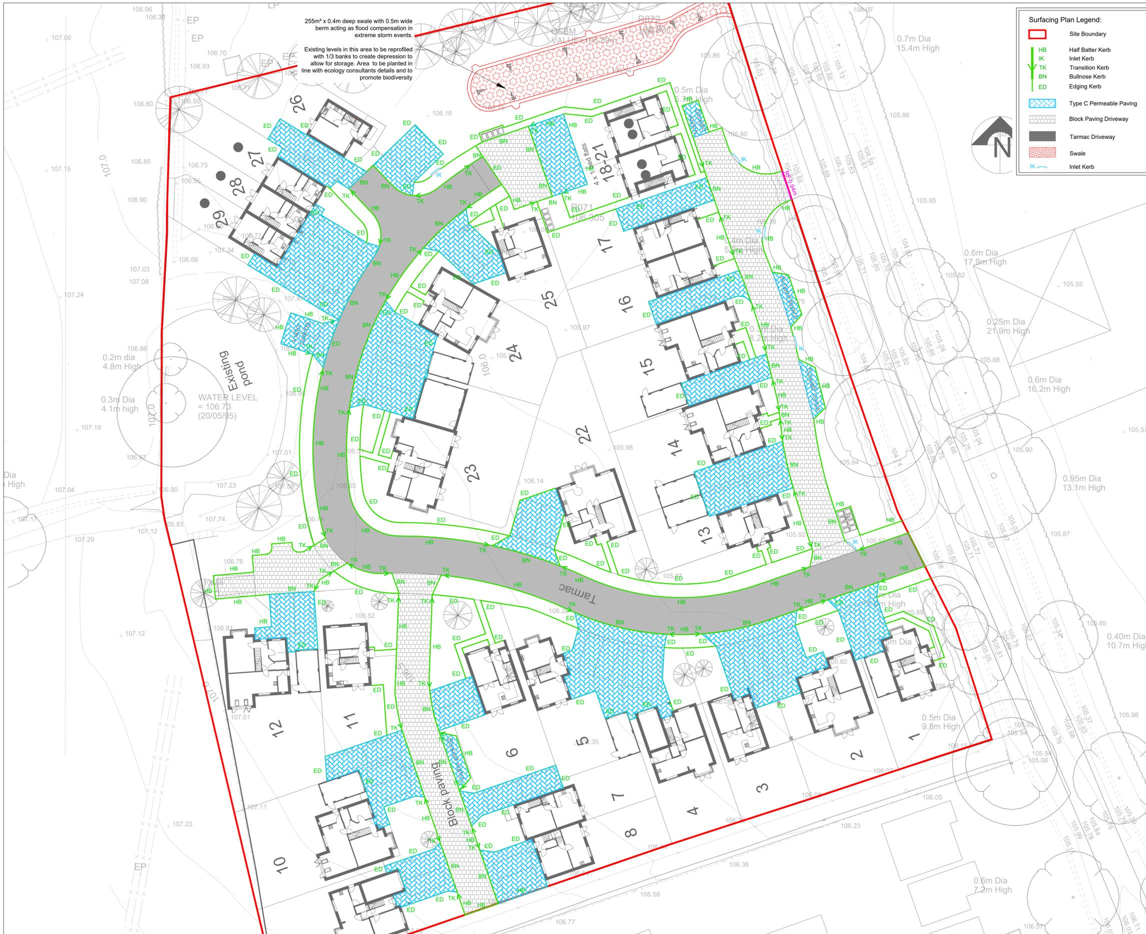
255m<sup>2</sup> x 0.4m deep swale with 0.5m wide berm acting as flood compensation in extreme storm events.
