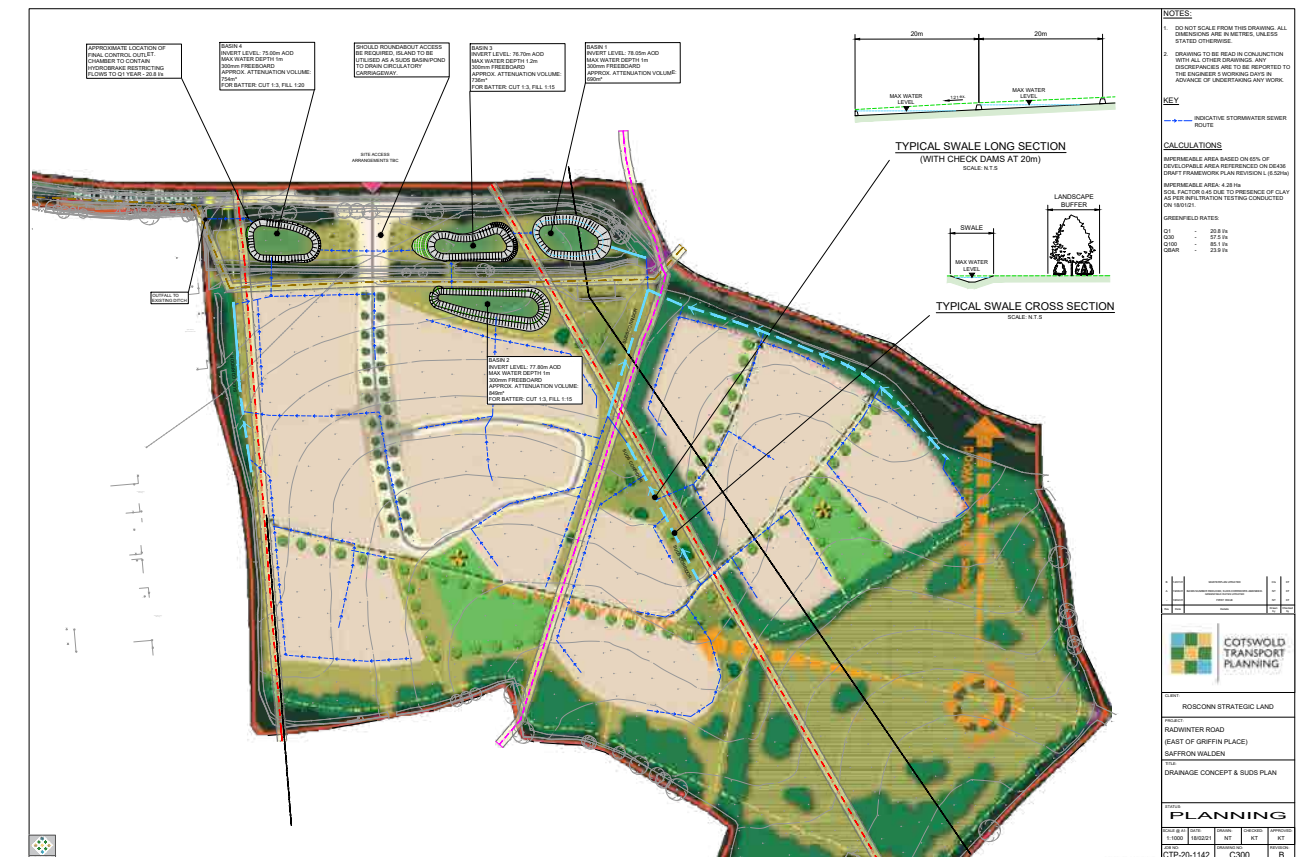
FIGURE 43 - DRAINAGE STRATEGY PLAN
