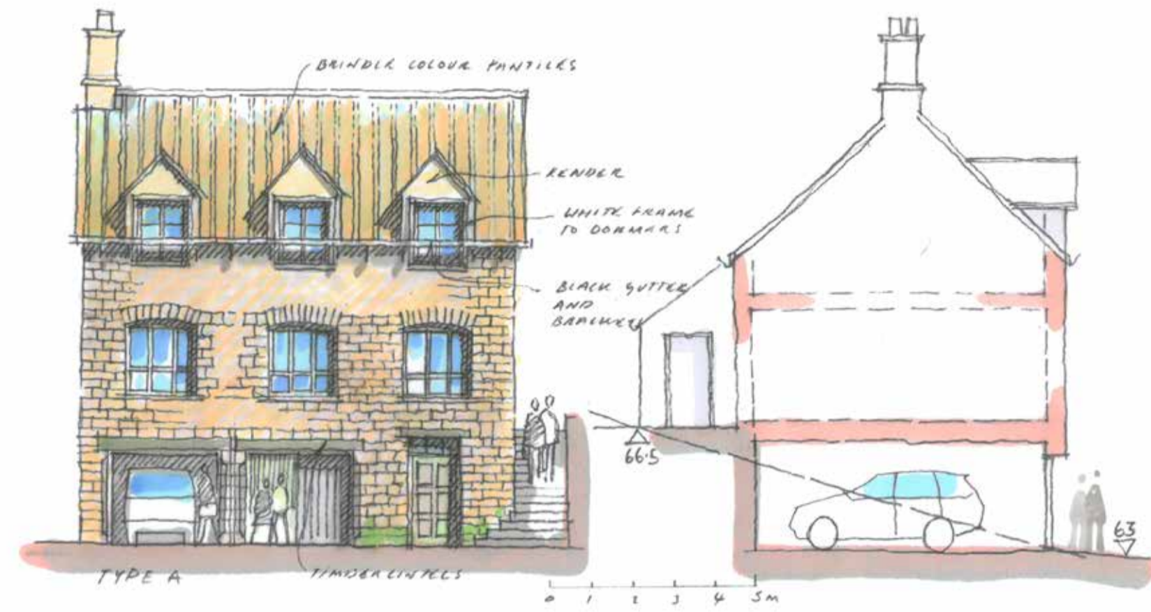
SPLIT LEVEL TYPE (UP-SLOPE)
