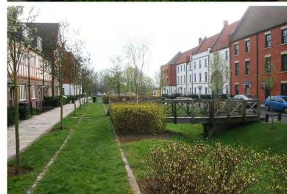
Broad Swales contribute to the site's SUDS network and enhance the central open space
